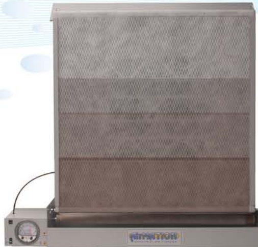
Auto-roll automatically indexes as particle build-up increases airflow pressure
